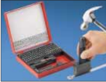
The impression is made by hitting the holder with a hammer.
